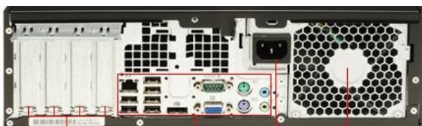
Expansion Slots Rear I/O Connectors Power In PSU Exhaust Fan
